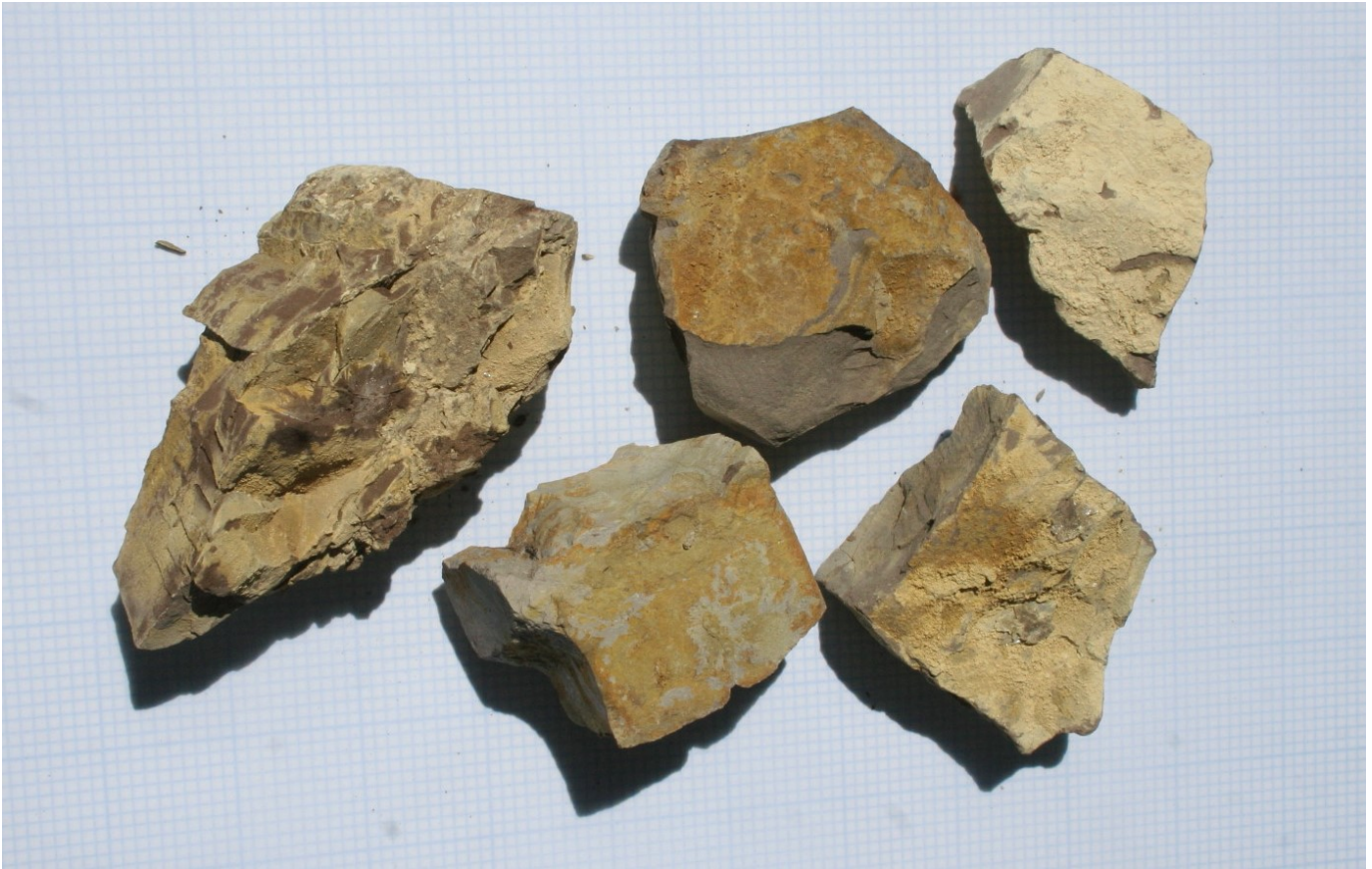
Jarosite is a basic hydrous sulfate of potassium and iron with a chemical formula of \text{KFe}_3+3(\text{OH})_6(\text{SO}_4)_2 . This sulfate mineral is formed in ore deposits by the oxidation of iron sulfides.
